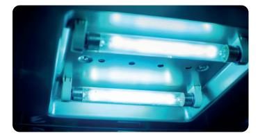
Ultraviolet (UV) light destroys microorganisms by targeting the DNA or RNA within microorganisms. This causes a photochemical reaction, creating abnormal links within the DNA or RNA. The chemical structure is distorted which interferes with the normal function of the microorganism, leading to mutations or inactivation.
