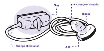
**Surface topography** refers to the physical features of a surface/device and includes complexities such as indentations, contours, textures, and any irregularities in shape. These complexities can block the light from reaching the surface beneath, causing shadowing. Most chemical products will not have an issue reaching these areas as additional attention can be paid by the user. Products such as foams may even get into surface scratches where pathogens reside.
