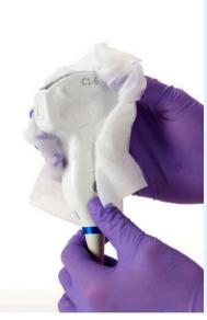
Wipe the surface of the probe in one movement to cover it with foam, as well as the holder, cable and plug, ensuring all areas come into contact with the Wipe.
