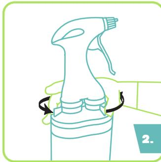
2. Fasten the levers anti-clockwise on each side of the trigger head to secure.
