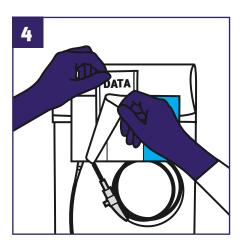
Peel the corner of the label and secure traceability data within the marked area. Reseal the pocket.
