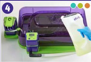
4 Add 5L of working solution into the Base.
