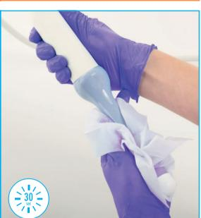
Wipe the probe holder, plug, cord, probe handle and probe shaft; ensuring all areas come into contact with the Wipe.
