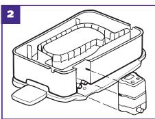
Apply a little amount of Lube lubricant onto the IQ drainage inlets. (See Section 5 Maintenance, Lubing IQ)
