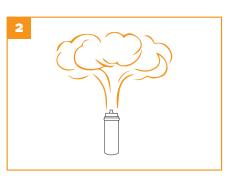
Place the bottle on an even surface and leave the room. Airstel forms a cloud that covers approximately 40m<sup>3</sup> in 1 minute (50ml bottle) and 150m<sup>3</sup> in 3 minutes (300ml bottle).
