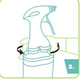
Fasten the levers anti-clockwise on each side of the trigger head to secure.
