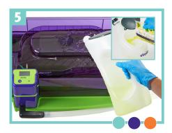
For the high-level disinfection cycle, add one sachet of Tristel Fuse for Stella to five litres of water and add to the inner compartment of the base.
