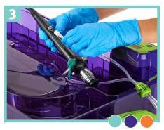
Add the cleaned medical device – connect lumened medical devices (in the case of Stella B/C) to Stella Pulse.
