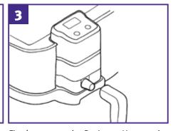
Firmly connect the Drainage Hose to the IQ and ensure the end of the tube is directed into a sink or waste container.
