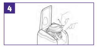
Replace the window, ensuring that the back ridge is pushed back correctly into Pulse and then fix the screw securely, taking care not to over tighten. *Pulse will not operate if the window is not replaced correctly.*
