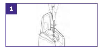
Ensure Pulse is turned off. Lift the green cover on Pulse. Using a flat head screwdriver, unscrew the clear window and remove it from Pulse.
