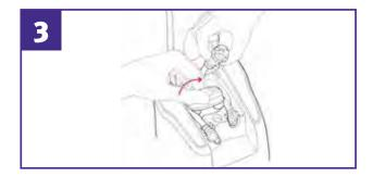
Insert the new Pump Hose into Pulse. Place the left-hand Pump Hose connector in first. This is the smaller connector with the plastic point. The hose then curves around the green pump head which can be turned by hand. Check that the hose is pushed down at the rear of the green pump head. The right-hand Pump Hose connector is then locked into place.
