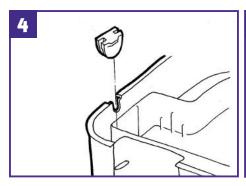
Apply the grommets into the tray cut-outs.
