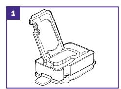
Once level, place the Base onto the Cradle. Stand the Lid in an upright position at the rear of the Base.
