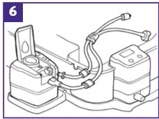
Remove the grommet nearest to the Pulse. Attach the Tube Set to Pulse by matching the male and female connectors. Place the green tube mount provided firmly on to the Base cut-out.
