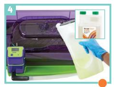
If using Stella for instrument cleaning prior to high-level disinfection, prepare five litres of Tristel Clean for Stella and add to the inner compartment of the base.
