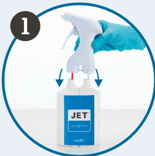
To assemble JET, take a trigger, unscrew the caps on the bottles, and following the **red A** and **blue B** indicators on the bottle label, insert the tubes into the respective bottle necks.
