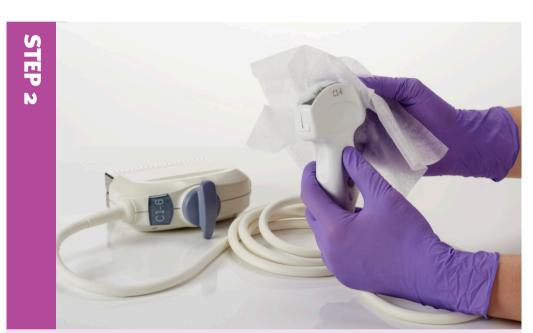
Use the wipe to spread the foam over the surface of the probe and ensure all areas are covered. Continuous wiping of the surface is not necessary and should be avoided to prevent shedding of the wipe.
